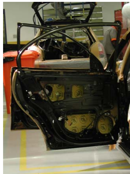
Figure 7. YellowGard® installed inside a door.
