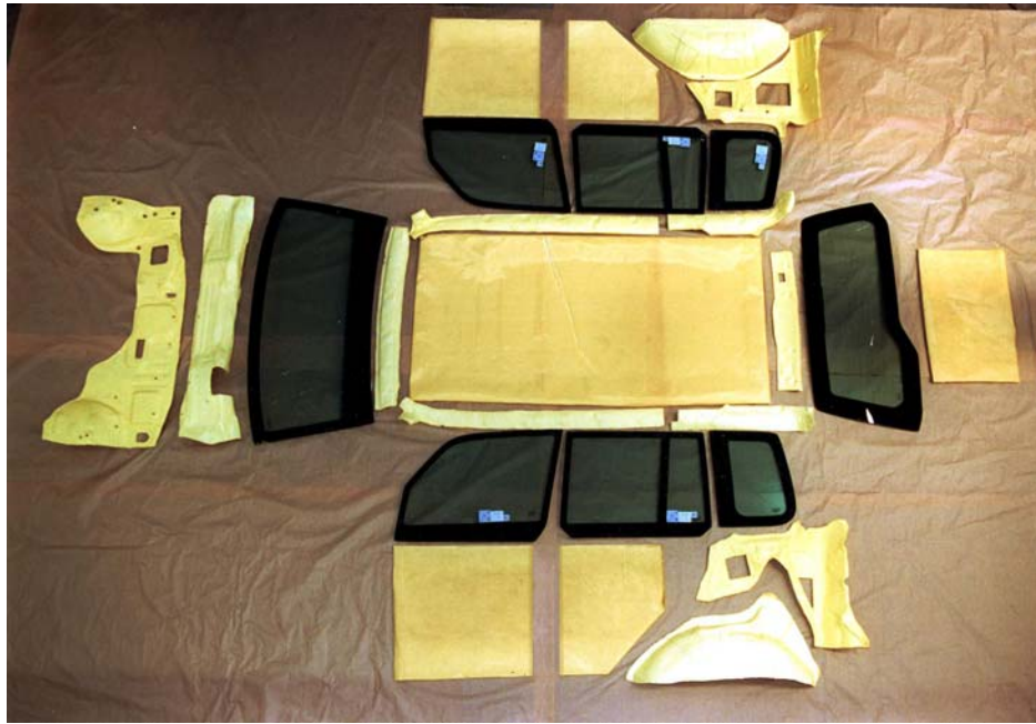
Figure 9. Assembly set of glazing and aramid ballistic panels for car armoring on line.
